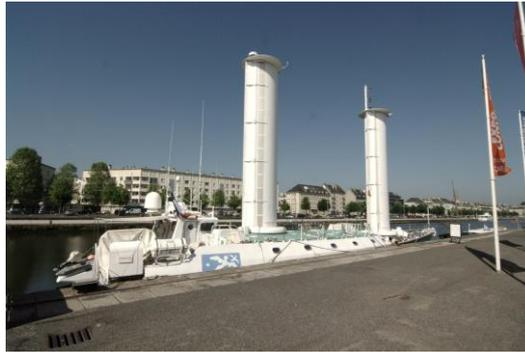
Figure 2. “Aleyone” of Cousteau equipped with Turbosails (picture by Entomolo).
